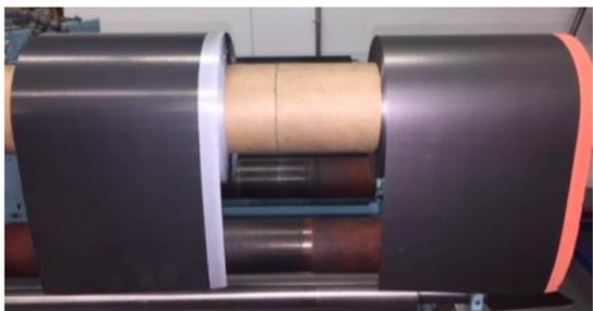
Figure 2. Dry battery electrode NMC roll (left) and graphite roll (right) double sided laminated onto current collectors, which is ready for cell assembly.
