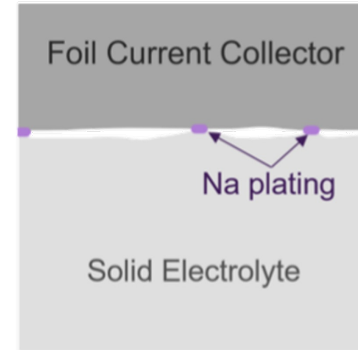
Poor interface contact
