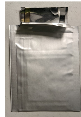
Single layer all-solid-state pouch cell
