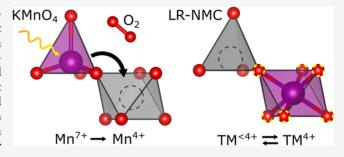
resulting in trapped molecular oxygen. For LR-NMC, we observe negligible evidence for Mn oxidation while stabilized tetrahedral sites correlate more with a reduced TM environment. Finally, the additional spectroscopic structures observed in oxidized oxygen RIXS for LR-NMC are absent for gas-phase molecular oxygen.
