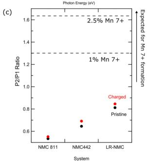
Figure 3. Mn K-edge spectra of (a) pristine and (b) charged states of LR-NMC, NMC 442, and NMC 811. The spectrum of KMnO<sub>4</sub> is also plotted, which exhibits a large pre-edge feature. (c) Pre-edge P1(t<sub>2g</sub>) and P2(e<sub>g</sub>) peak intensity ratios are plotted. Horizontal lines indicated predicted peak ratio for 1% and 2.5% Mn<sup>7+</sup>. Information on peak ratio predictions can be found in the Supporting Information.
