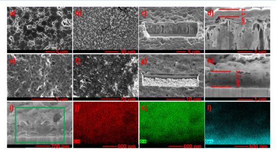
**Figure 2.** SEM images of LMC coated Cu foil. (a, b) Top view and (c, d) cross section view of Cu after 2 h of Li deposition at 0.5 mA cm<sup>-2</sup> in 0.2 M LiI-EC/DMC electrolyte. (e, f) Top view and (g-i) cross section view of Cu after 2 h Li deposition at 0.5 mA cm<sup>-2</sup>, then stripped to 1 V in 0.2 M LiI-EC/DMC electrolyte. (j-l) EDS elemental mapping of carbon, oxygen, and copper in part i, respectively.
