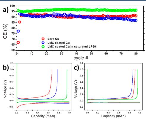
Figure 4. (a) Coulombic efficiency comparison of LillCu cell cycled in LP30 electrolyte at 0.5 mA cm<sup>-2</sup> for 1 mAh cm<sup>-2</sup>. (b) The first cycle voltage profiles. (c) The 80th cycle voltage profiles. (Red, bare Cu; blue, LMC coated Cu; green, LMC coated Cu in LMC saturated LP30.)
