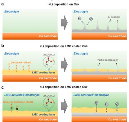
solvents. The solution dynamics of these key SEI components directly affects the stability, composition, and microstructure of
