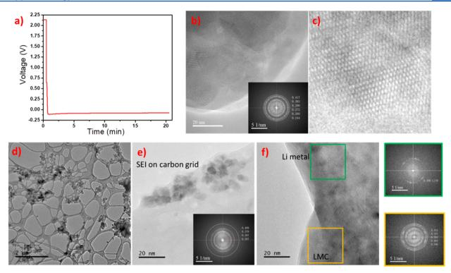
Figure 1. (a) Voltage profiles of Li plating on lacey carbon grid in 0.2 M LiI-EC/DMC electrolyte, 0.5 mA cm $^{-2}$  for 20 min. (b, c) Cryo-TEM images of the LMC powders from the reaction between LiI and DMC. (d-f) Cryo-TEM images of the Li from the 0.2 M LiI-EC/DMC electrolyte after 20 min deposition at 0.5 mA cm $^{-2}$ .
