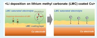
which improves the Li plating/stripping Coulombic efficiency from 90.5% (bare Cu in commercial electrolyte) to 96.1% at 0.5 mA cm<sup>-2</sup> and 1 mAh cm<sup>-2</sup>.
