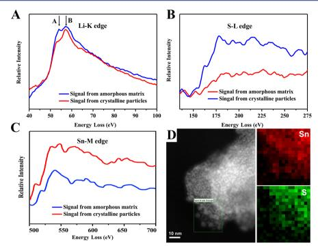
Figure 4. (A) Li K-edge, (B) S L-edge, and (C) Sn M-edge results for SnS<sub>2</sub> nanocrystals lithiation reaction in different phases. (D) EELS mapping results showing that the formed particles are Sn-enriched and the amorphous phase is S-enriched.
