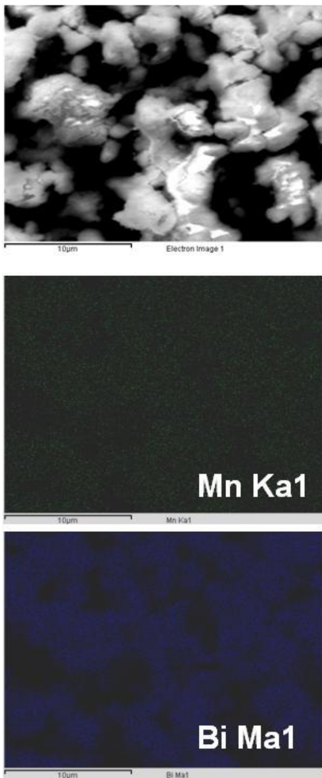
Figure 6.7. \text{Bi}_2\text{O}_3 particle after soaking in 12 ml Of aqueous 2M \text{Mn}(\text{NO}_3)_2 solution. Top: SEM image of the EDS site. Middle: EDS mapping using the Mn L_{\alpha 1} data. Bottom: EDS mapping using the Bi M_{\alpha 1} data
