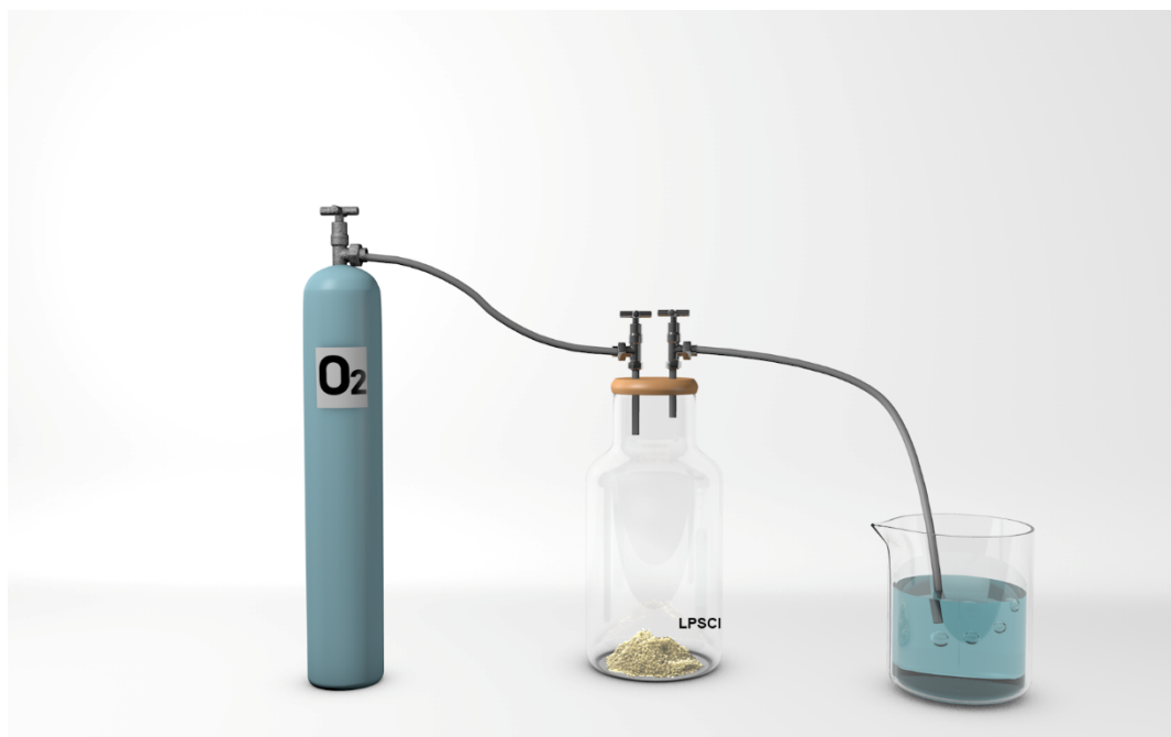
Figure D.6. Setup for purging oxygen to oxidize LPSCI to form oLPSCI
