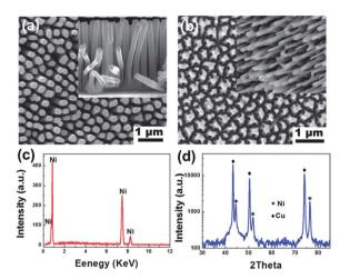
**Fig. 1** Plan-view SEM images of the (a) as-grown and (b) electropolished Ni nanowire arrays. The corresponding side-view images are in the insets; (c) EDX spectrum of the electropolished sample; (d) XRD  $\theta$ -2 $\theta$  scan of the electropolished Ni nanowire arrays on a copper substrate.
