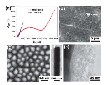
**Fig. 5** (a) Nyquist plots of the Ni–Si nanocable and Si film electrodes at the potential of 2 V during the charging process. Plan-view SEM images of those two electrodes taken after delithiation (b) thin film; (c) nanocable. TEM images taken from the nanocable sample after delithiation (d) low magnification; (e) high magnification.
