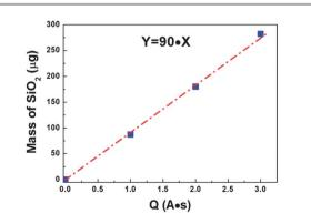
Fig. 3 Linear dependence between the mass of  $SiO_2$  and the quantity of charge passed through the electrode during electrodeposition of Si.
