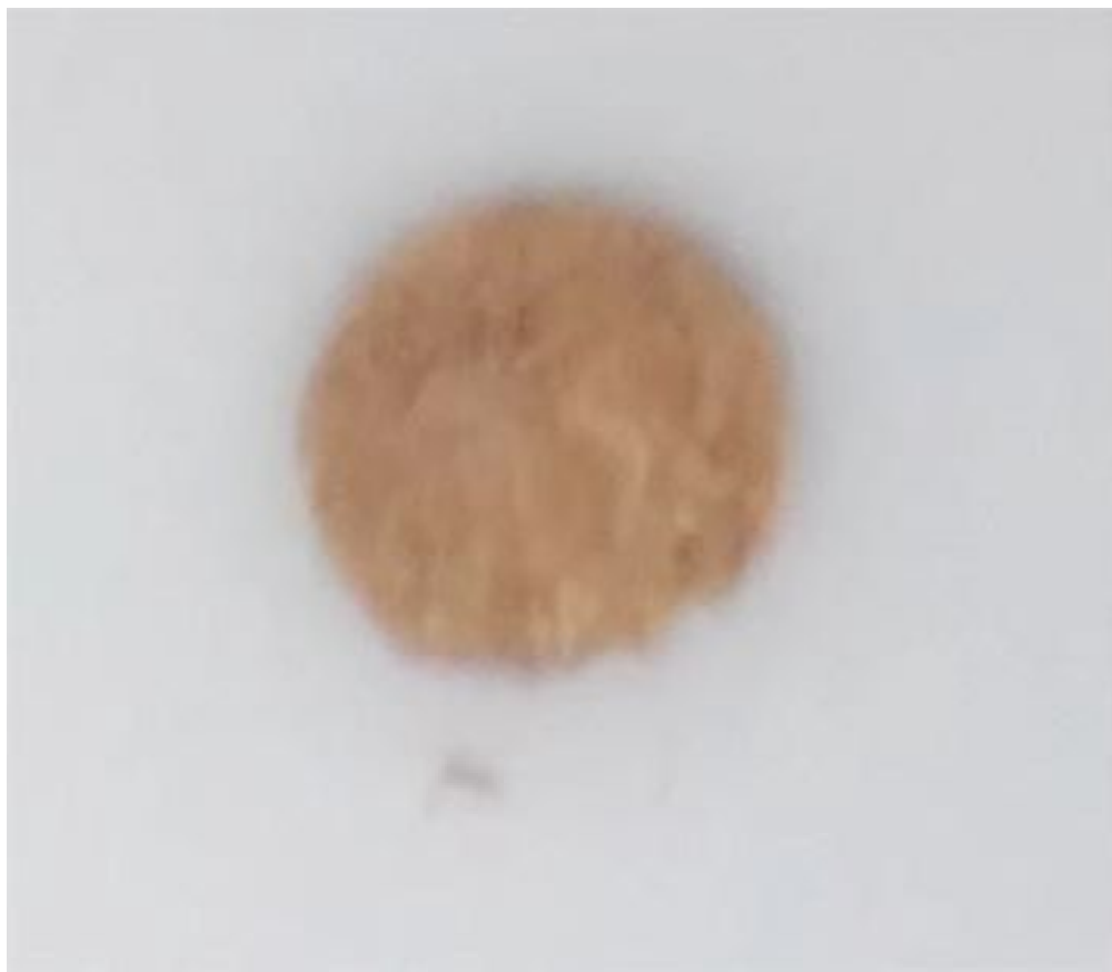
Figure 7.6: Optical photo of lithium metal after 21 days of reaction with fluoromethane under an applied 1200 psi of pressure.
