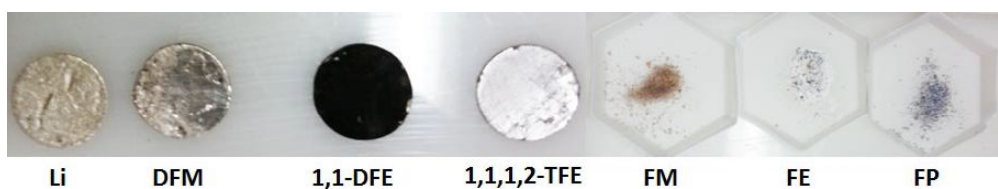
Figure 7.1: Optical images of reaction products resulting from chemical reduction of fluorinated solvents with lithium metal.
